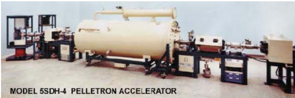
*Fig. 3 Photograph of the National Electrostatics ion accelerator. The dual ion sources are seen at left. The large tank contains the pellet charging chain and terminal. The analyzing magnet is at the right.*
